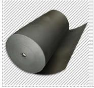
heat and impact sound insulating mat with a thickness of 5 mm, permanently elastic and pressure-resistant, can be double fitted (pay attention to traffic loads!), impact sound improvement when single fitted of up to 20 dB, when double fitted of up to 22 dB,  $\lambda$  = approx. 0,041 W/ (m·K), (width = 1500 mm, thickness = 5 mm)
