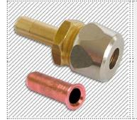
pipe socket ø 8 mm upon compression fitting ø 8 mm, flat sealing with rubber ring (incl. 1x supporting sleeve)
