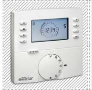
230 V, 50 Hz, relay / closer, scale 5...30°C, time-dependent valve control, suitable as master for master-slave-operation, background lighting, pure white
