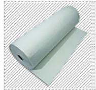
sound reducing, thin insulation layer, especially suited for retrofit, when only low floor building heights are possible, impact sound improvement of up to 21 dB,  $\lambda$  = approx. 0,040 W/ (m·K), (width = 1250 mm, thickness = 4 mm)
