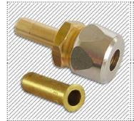
pipe socket ø 10 mm upon compression fitting ø 10 mm, flat sealing with rubber ring (incl. 1x supporting sleeve)
