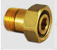
screw connection 3/4" for the connection of submanifolds resp. single plug connectors to conventional manifolds and valves, consisting of union nut G 3/4" euro cone with o-ring sealing and sleeve R 1/2"
