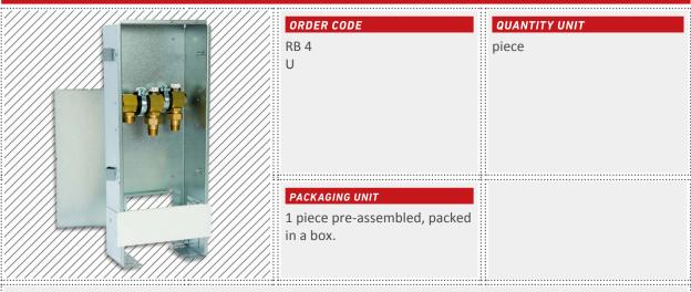
as sub-distribution without thermostatic valve and limiting of the return temperature for use within premixed underfloor heating loop, built-in box with cover ready to decorate and tile, closed, uncontrolled with ventilation valve, for areas of up to 16 m<sup>2\*</sup>
