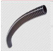
for heating pipe Ø 10 mm corrugated pipe, length = 300 mm, for the mechanical protection of the heating pipe wherever the pipe comes out of the floor system and in areas of leadthrough (e.g. professional joints)
